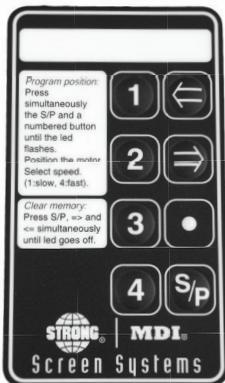
For your safety, these units will not operate until a minimum of two stops are programmed.
