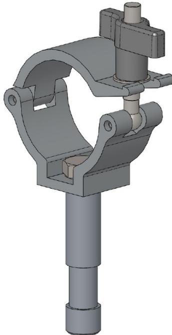
Super Lightweight Beamer Clamps consist of a 16mm beamer spigot fixed to a Super Lightweight clamp. Beamer clamps are commonly fitted into a receiver mounted on a stand. Once the clamp has been inserted into the receiver and locked in to place the barrel or truss can fitted into the clamp following the instructions set out in Sections 10d to 10h.
