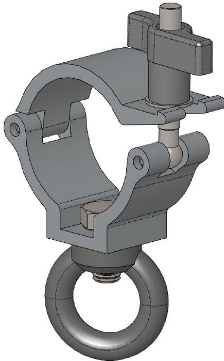
Hanging clamps are commonly used to secure rope directly or via shackles, karabiners, hooks etc.
