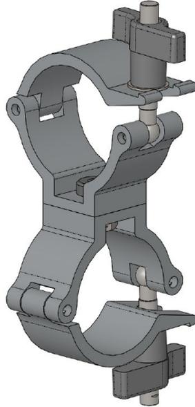
These couplers are used for rigging two sections of truss or barrel together. The couplers consist of two Super Lightweight clamps bolted together and are free to rotate relative to each other. To install, attach each of the clamps that comprise the coupler to their respective barrel or truss following the instructions set out in Sections 10d to 10h.
