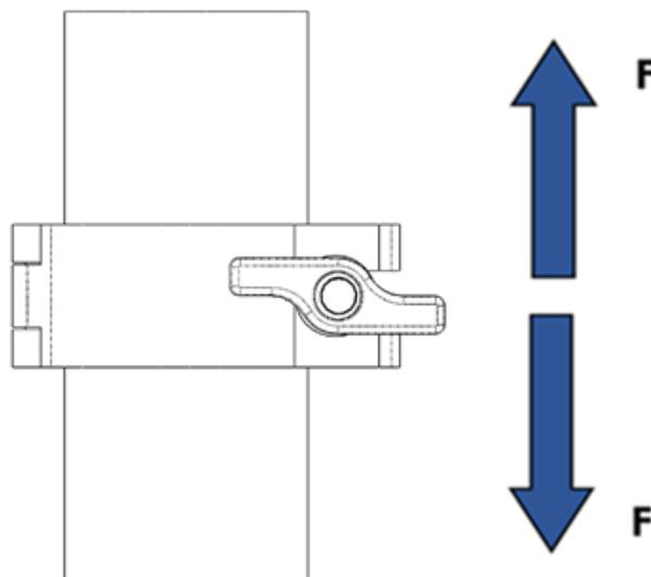
⚠ Do not use fixings that, when tightened, will contact the tube or barrel on which the clamp is fixed as highlighted above.
